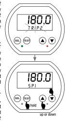
Note that the unit will not respond to changes in temperature, LEDs are turned off, and the alarm relays will maintain their prior states while the TEST button is held.
