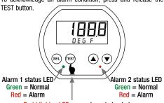
Red blinking LED = unacknowledged alarm Press Test to acknowledge blinking alarm
