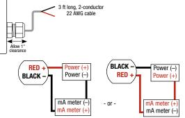
If the 4-20 mA analog output is not required, the transmitter will function as a low voltage powered temperature indicator when connected to any 8 to 32 VDC power supply. Connect the loop (+) supply to the RED lead and the loop (-) supply to the BLACK lead.
