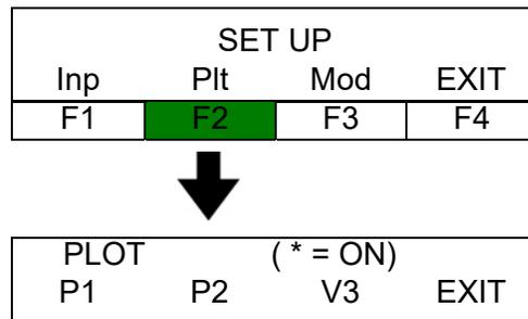
Pressing a function key from the PLOT screen toggles the plotting on and off for that channel.
