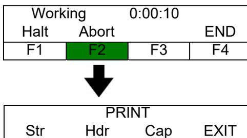
Pressing the F4 key from the Working screen stops the recording and proceeds to saving the recording.
