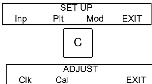
Pressing the F1 key from the ADJUST screen allows the user to change the time setting on the internal clock.
