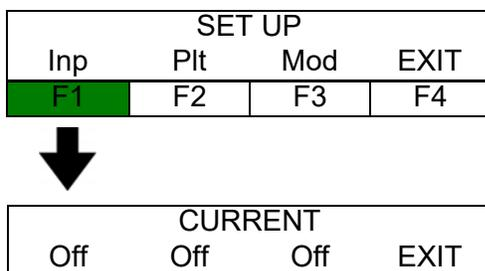
Pressing the F1 key from the CURRENT screen toggles between the 5 available inputs for channel 1.
