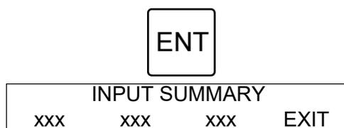
The INPUT SUMMARY screen displays what type of recording is stored on the three channels.
