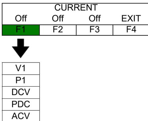
Pressing the F2 key from the CURRENT screen toggles between the 2 available inputs for channel 2.
