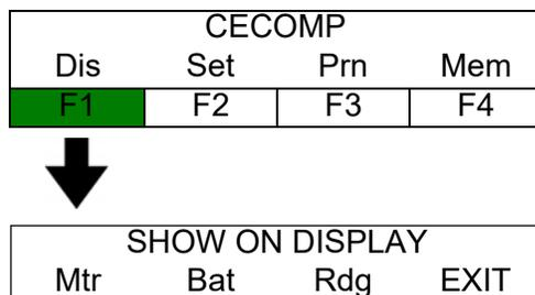
The SHOW ON DISPLAY menu allows the user to utilize the real-time meter capabilities of the TriScan 2+, view the battery charge level, display previously stored recordings by single stepping through memory or by entering discrete recording numbers or return via EXIT to the main menu.
