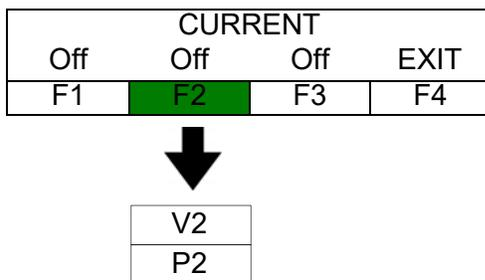
Pressing the F3 key from the CURRENT screen toggles between the 2 available input for channel 3.
