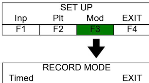
Pressing the F1 key from the RECORD MODE screen toggles between the timed and continuous mode.
