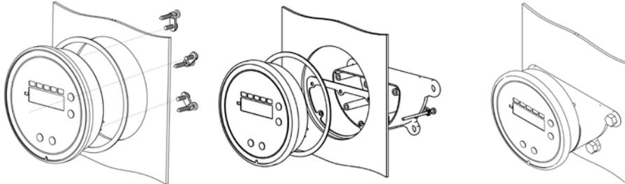
**Flush Mounting** – For new applications, cut a 4 9/16" diameter hole in the panel. Insert the gauge with the provided gasket through the hole and secure it to the panel with the provided mounting tabs and screws. They fit in industry standard holes ranging from 4 9/16" to 4 13/16". Simply remove the old device and insert the new gauge into the existing cutout.
