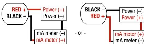
To use the transmitter as a low voltage powered gauge connect it to any 8-32 VDC power supply.
