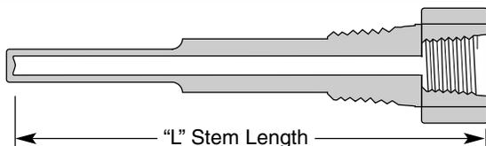
NOTE: Some thermowell manufacturers refer to stem length as dimension "A" or "S". It is NOT the same as thermowell insertion length.
