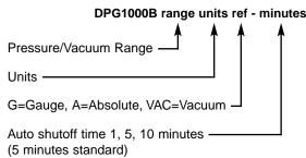
Example: DPG1000B100PSIG-5 = DPG1000, Battery powered, 100.0 psig, 5 minute shutoff
